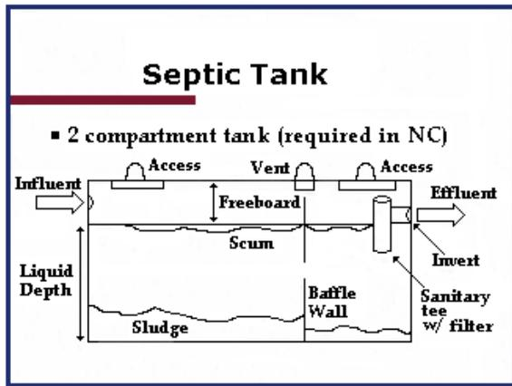
A **conventional** septic system consists of a **septic tank** (above), a **distribution box**, and **nitrification lines** all connected by pipes called **conveyance lines**. All of these components are designed to be resistant to corrosion. The wastewater first flows into the septic tank where heavy solids and lighter scum separate in a process known as **primary treatment**. Some of the scum and
