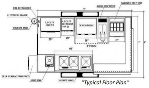
\*\*Floor plans must be accurate and drawn to scale: 1/4 inch=1 foot is required
